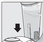
**1** Rinse and fill the **water container** with fresh cold water. Turn on the machine by pressing the **on/off switch**. Open the **brew mechanism**. Opening the **brew mechanism** will initiate the heating of the water and the **HEATING** light will flash.
