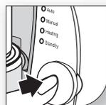
**4** When the **AUTO** light illuminates, press and release the **start/stop button**. Brewing will start automatically. There may be a short pause during brewing; this is normal. The **AUTO** light flashes throughout the brew cycle. When the machine has finished brewing, the indicator light will move from **AUTO** to **MANUAL** and then, after a delay of 30 seconds, to **HEATING**.
